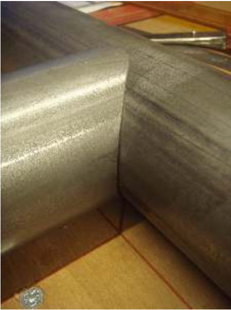
Profiled tube ready for welding
